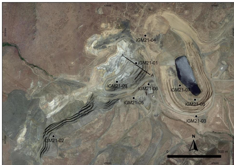
Figure 2 – Surface Plan of the 2021 Drill Program Targeting Open Pit Mineralization
