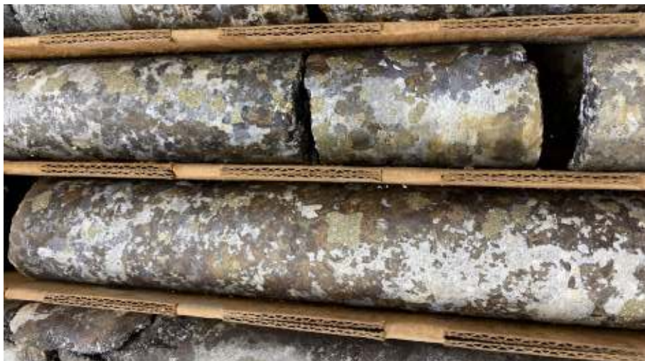
Figure 4 – Core from iRH22-43 showing massive sphalerite (brown), galena (gray) and pyrite (yellow)
