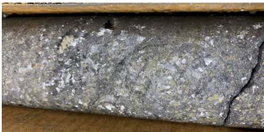
Figure 4 – Core from iRH22-43 showing massive sphalerite (brown), galena (gray) and pyrite (yellow)
