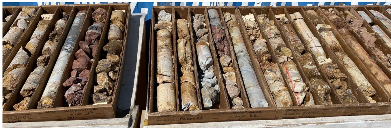
Oxidized, faulted, and argillized Panther Canyon (PG20-03)
