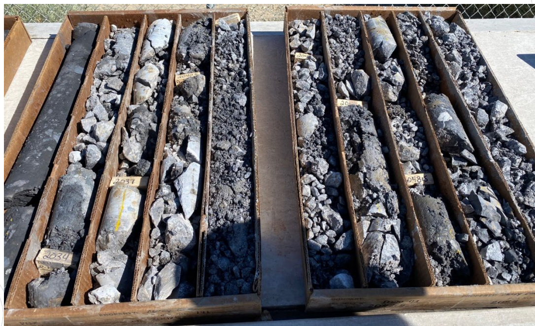
Strong decarbonatization of Favret and Dixie Valley in a fault zone (PG20-03)
