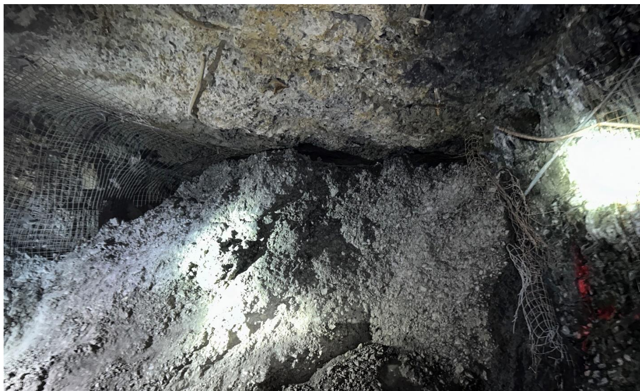
Photo 16-2: Cemented Rock Fill in Adjacent Cut
