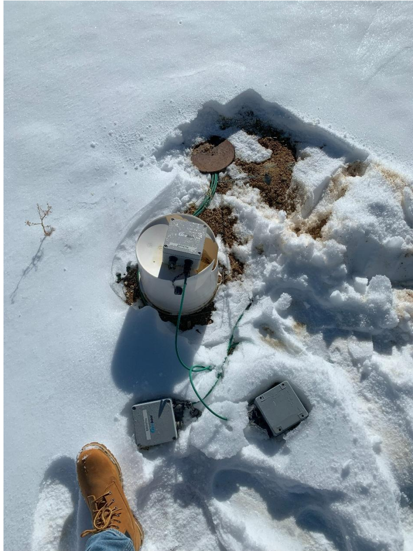
Figure 11: Collar Location of Drill Hole with Brown Top Casing and Piezometer
