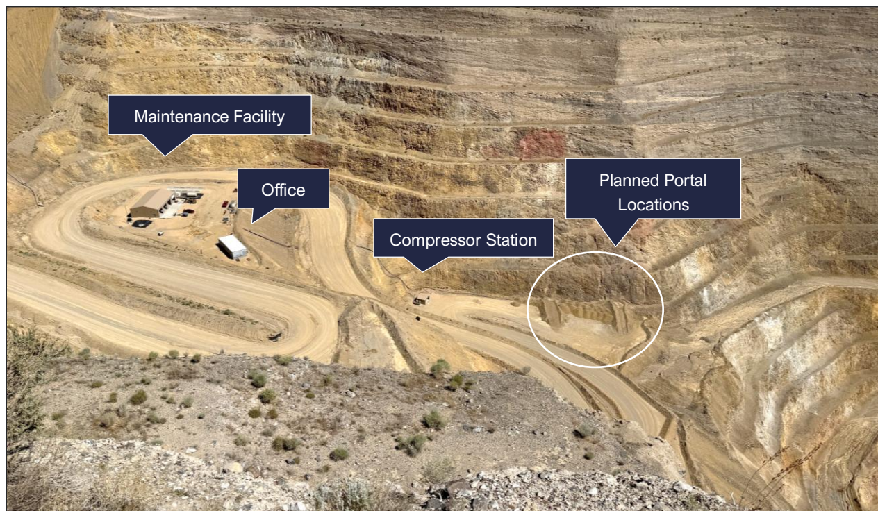
Figure 4: Overview photograph of the Archimedes underground planned portals and surface facilities.
